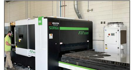
*The sheet metal shop's laser cutter is at least twice as fast as the plasma cutter.*
