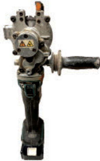
The Makita Rebar Cutter is a much safer tool to use than a Partner Saw when cutting rebar that is not at ground level.
