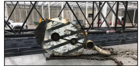
The crane block
